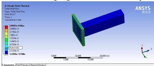
Figure 8. Heat flux concerning SSF aluminum pin fin
