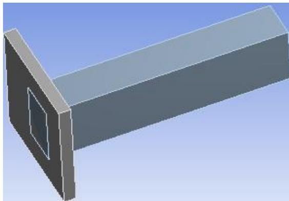
Figure 2. CAD model of SSF pin fin
