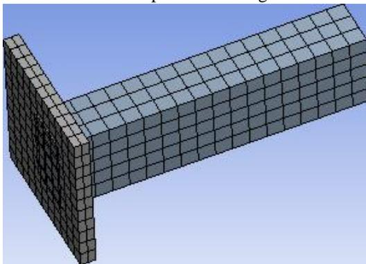
Figure 3. SSF pin fin computational mesh
