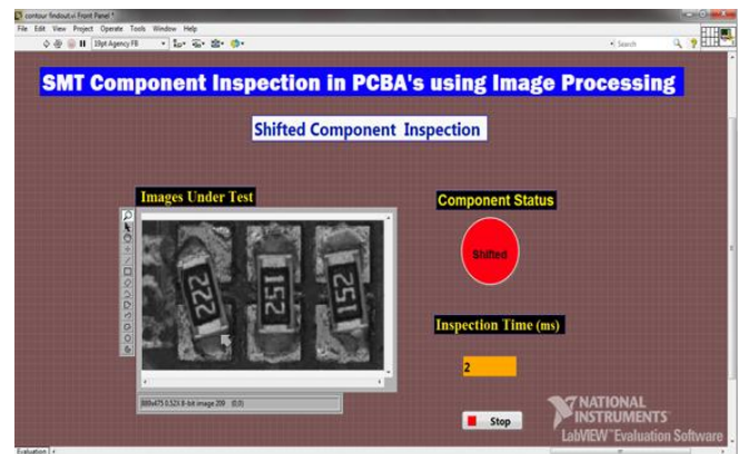
Fig 5: Status indication of defective image using Contour Analysis technique
