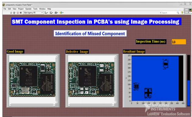
Fig 17: Front panel window of Pixel subtraction for Sample 2 Images
