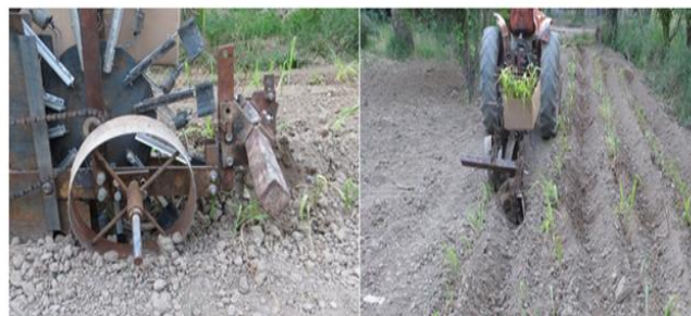
Fig.3: Field performance evaluation of the semi-automatic field crop transplanter
