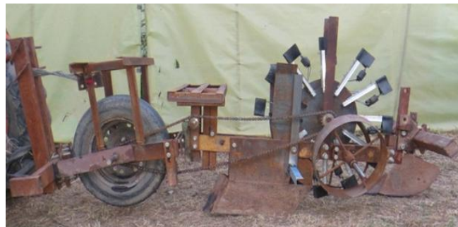
Fig.2: The assembled prototype of the semi-automatic field crop transplanter
