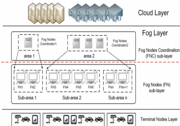
**Fig 1. Terminal Nodes enabled FoG Computing Architecture**
