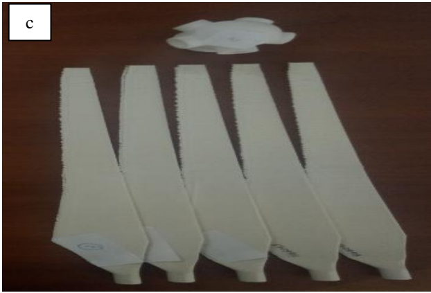
Fig. 15. Optimized Blade & Hub Manufactured by 3D Printer (a) Blade=3, MK115 airfoil (b) Blade=3, Naca 2412 (c) Blade=5, SG 6043 airfoil
