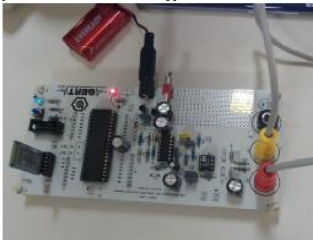
Figure 5. Signal acquisition circuit for ECG electrode
