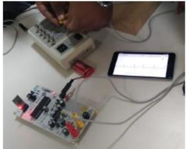
Figure 7. Prototype setup for ECG signal Acquisition from the MWCNTs/PDMS composite electrode.
