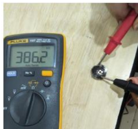
Figure 3. Resistance of the proposed electrode
