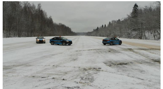
Fig. 3. Coordinated turning of convoy comprised of three Lada Vesta vehicles.
