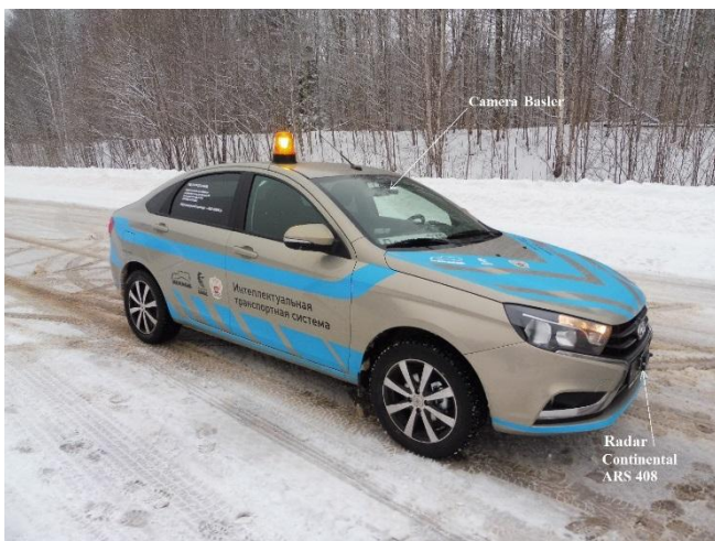
Fig. 1. Lada Vesta equipped with Continental ARS408 radar and Basler video camera.
