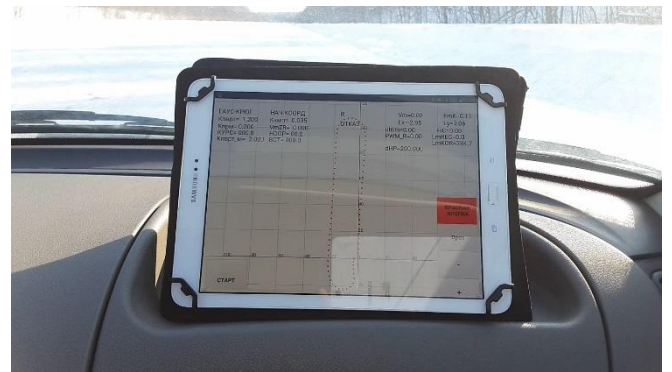
Fig. 4. Data input display of master manned vehicle showing motion path.
