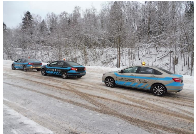
Fig. 2. Unmanned Lada Vesta vehicle convoy with manned master vehicle at starting position of Dmitrov test track.
