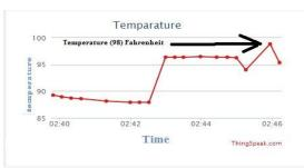
The temperature data which is in the Celsius scale will have been converted into the Fahrenheit scale using MATLAB. So, our retrieved data for temperature remains in Celsius scale. The following figure shows the temperature rise with a human touch and goes back to room temperature once contact is removed along with the time of entry.
