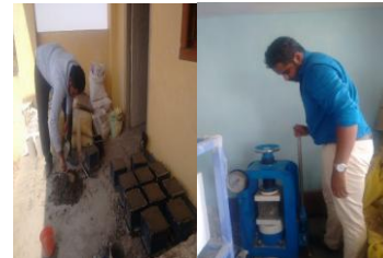
Figure 10: Cubes Casting and Testing
