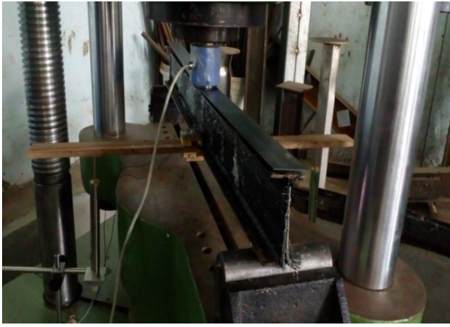
Fig. 4. Experimental setup showing Three Point Loading
