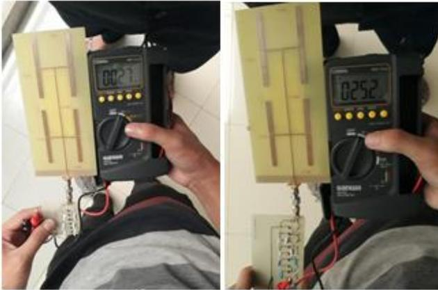
**Figure 11: Indoor RF Energy Harvesting Test**
