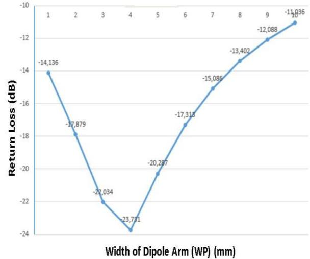
Figure 4: Variation of Return loss on the Dipole Arm Width
