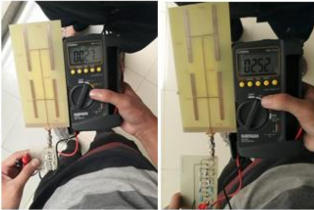
Figure 11: Indoor RF Energy Harvesting Test Left: with 3-stage rectifier, Right: with 7-stage rectifier
