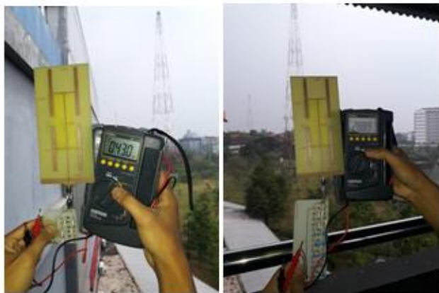
Figure 12: Outdoor RF Energy Harvesting Test Left: with 3-stage rectifier, Right: with 7-stage rectifier
