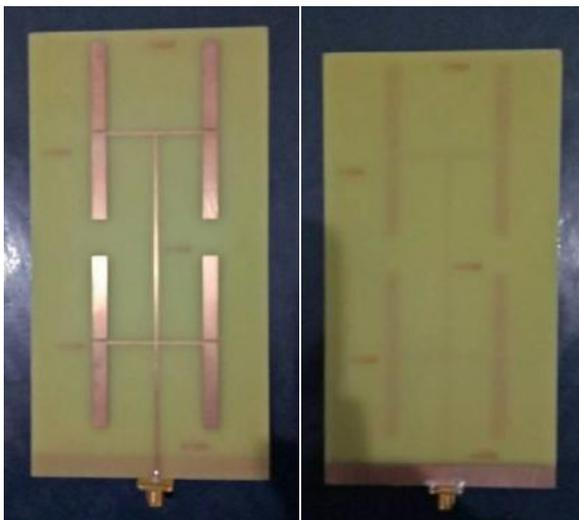
Figure 8: The Fabricated Antenna
