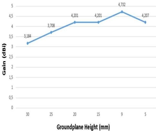
Figure 3: Variation of Gain on the Groundplane Height
