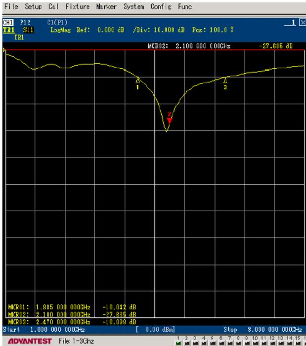
Figure 7: Measured Return Loss of the Proposed Antenna
