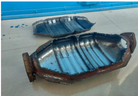
Figure 1: Existing Catalytic Converter
