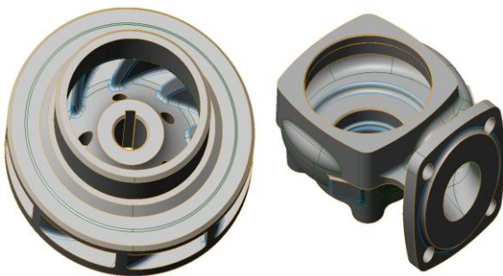
Fig.3. Solid geometry of pump impeller and casing
