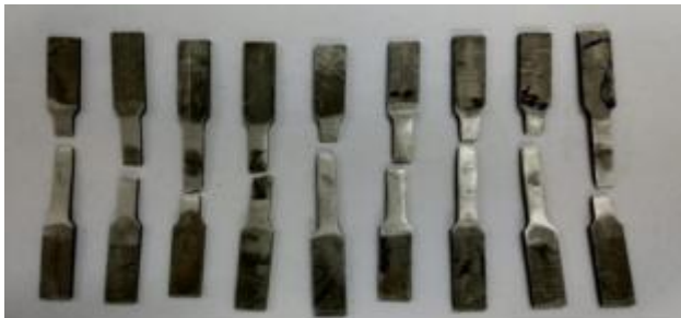
Fig. 6 Tensile specimen after the experiment
