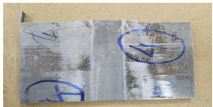
Fig. 3 FSW joint with hardness indentation
