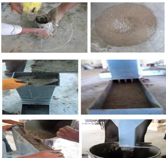
Figure 1: (a) Slump cone, (b) L-Box, (c) V-Funnel
