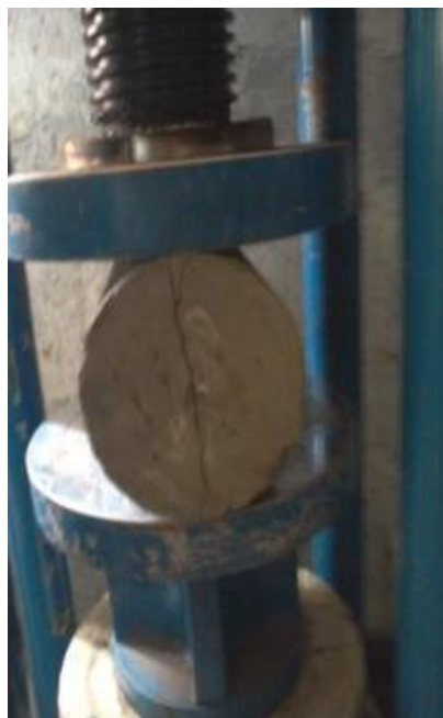
Fig-2 Split tensile strength test
