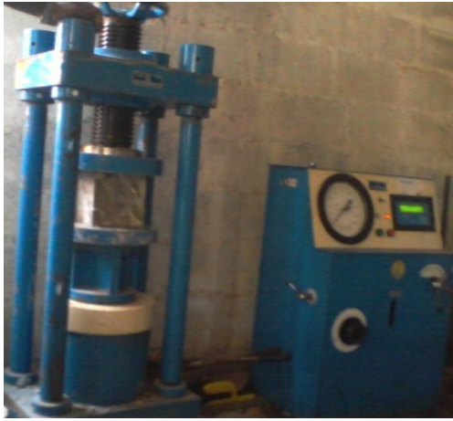
Fig-3 Compressive strength test
