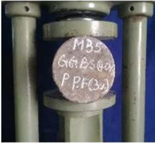
Figure 3 Cylinder Split Tensile Strength test results for M35 grade with 40% of GGBS (b) 3% of Polypropylene fibre in HPC
