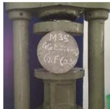
Figure 3 Cylinder Split Tensile Strength test results for M35 grade with 40% of GGBS (a) 0.3% of Glass fibre in HPC
