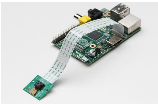
Fig 10 Camera interfaced with raspberry Pi Module
