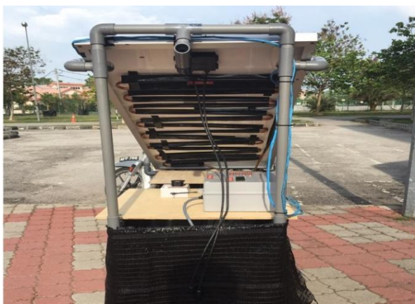
Fig. 3 (b) Back view of PVT water collector
