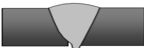
Fig. 4 Incomplete root fusion
