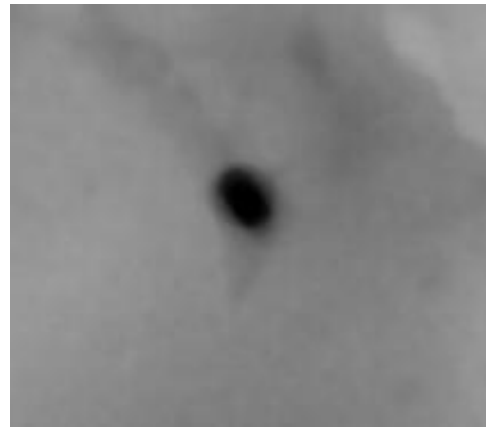
Fig. 6 Original image before enhancement and blow hole weld defect
