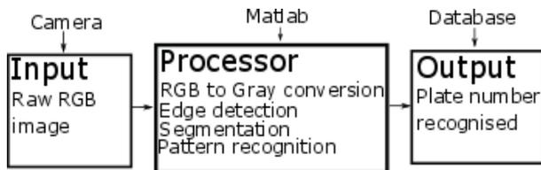
Fig. 14 Block diagram
