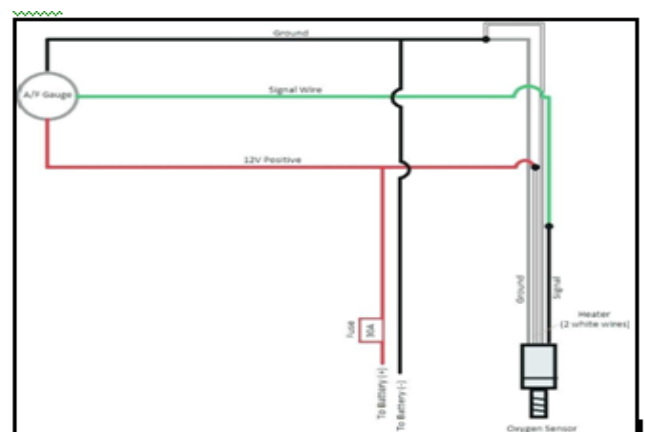
Fig. 2 wiring diagram of the oxygen sensor to the AFR meter
