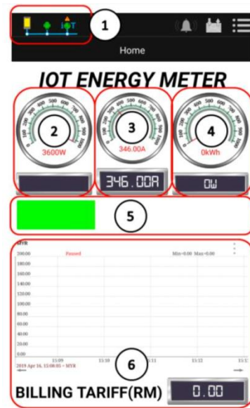
Fig. 7 Virtuino apps which also linked to Thing Speak energy data consumption visualisation for IoT
