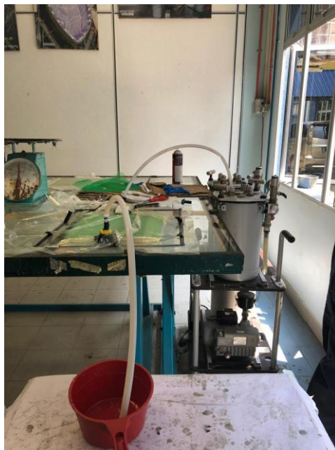
Fig. 2 Vacuum Infusion Setup
