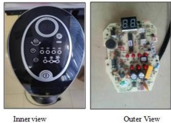
Fig. 19 Old control board
