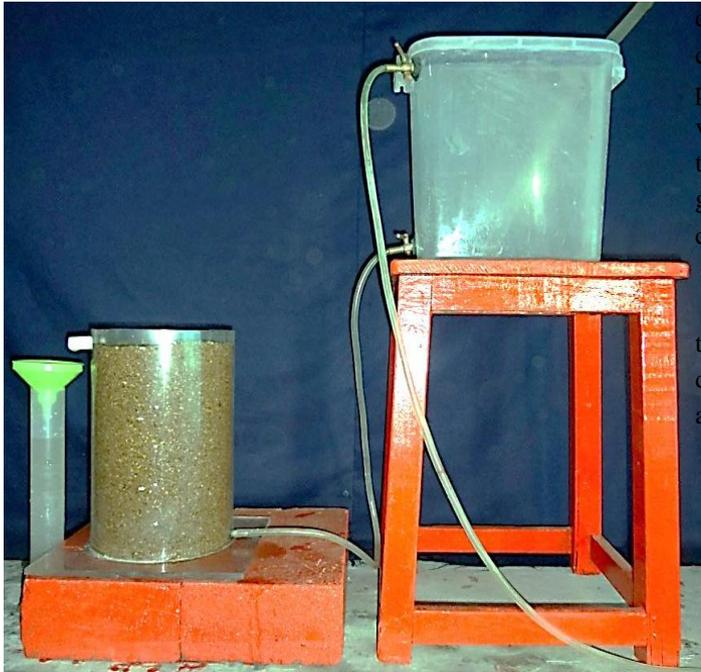
Fig 2 Hydraulic Conductivity typical test setup
