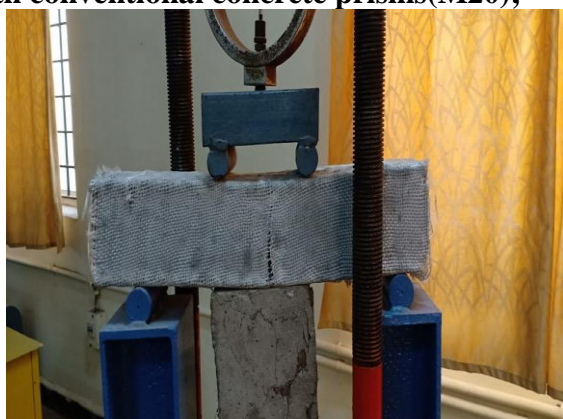
fig 8 images showing the bending moment while doing flexural test
