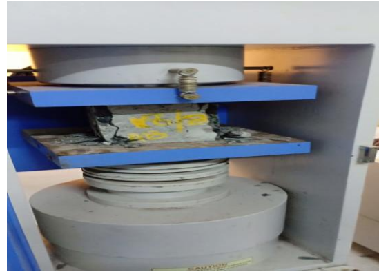
Fig 3 COMPRESSIVE STRENGTH TESTING ON CUBE.
