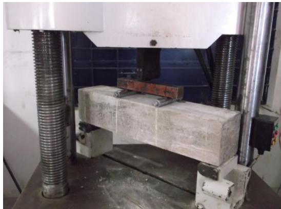
Fig 2: Flexural strength test of concrete
