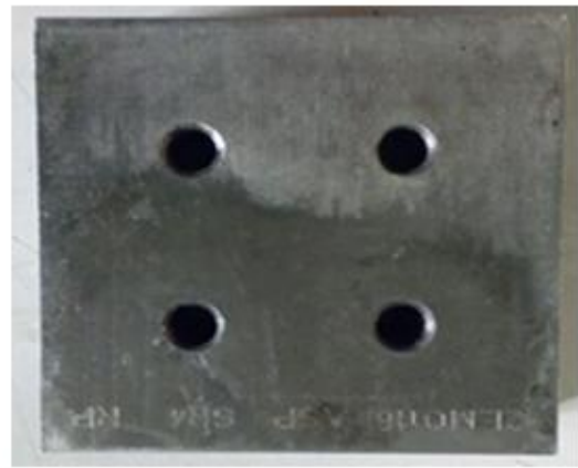
Fig 17 New tool developed using S7 material
