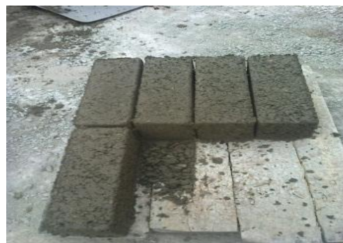
Fig. 3 Let the Bricks dry for at least one week.
