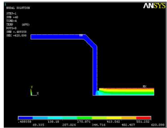
Figure 8 Screenshot of Nodal temperature for rib width of 8mm bogus of fashioned iron
