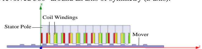
Fig. 3. 2-D axial symmetric finite element model of tubular linear switched reluctance actuator.
