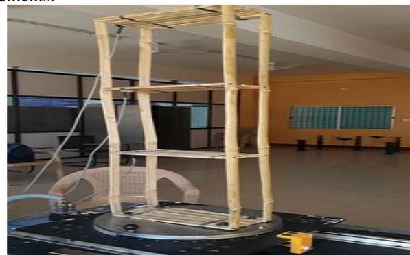
**Fig.2: Shake Table with Bamboo Model**
