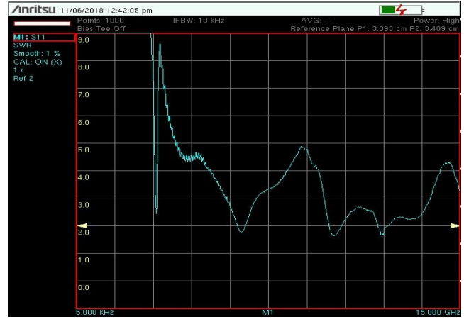
Fig 15 Measured VSWR for Proposed Multi Band Octagonal Patch Antenna Model
