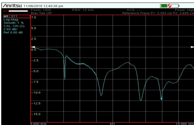
Fig 14 Returnloss for Proposed Multi Band Octagonal Patch Antenna Model
