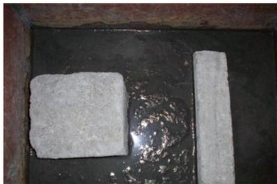
**Plate 3. 10% fly ash + lime modified marginal soil sample after liquefaction at frequency of 0.53 cycles/sec**
