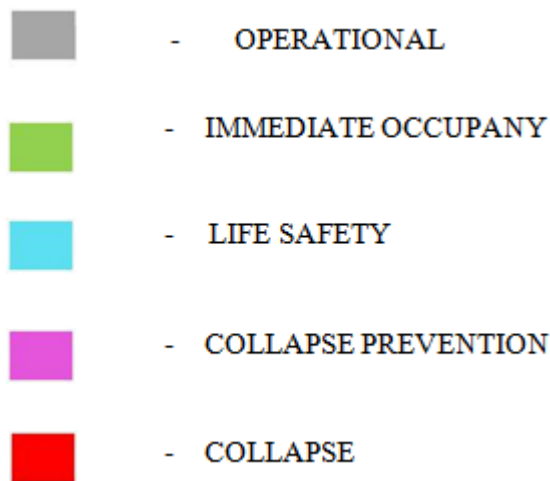
Figure 14 Different Stages in Performance of Buildings
