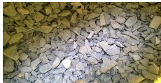
Fig. 1 Crushed kadappa Waste
