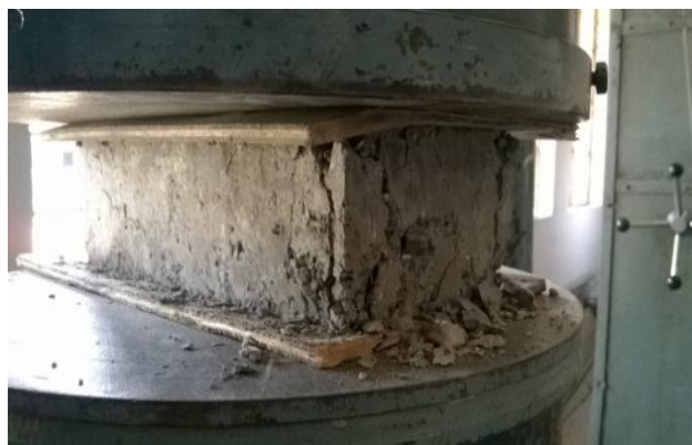
Fig. 4 Failure of KFB
