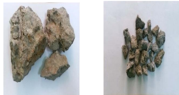
Before Processing After Processing Fig. 3 Course Aggregate Materials
