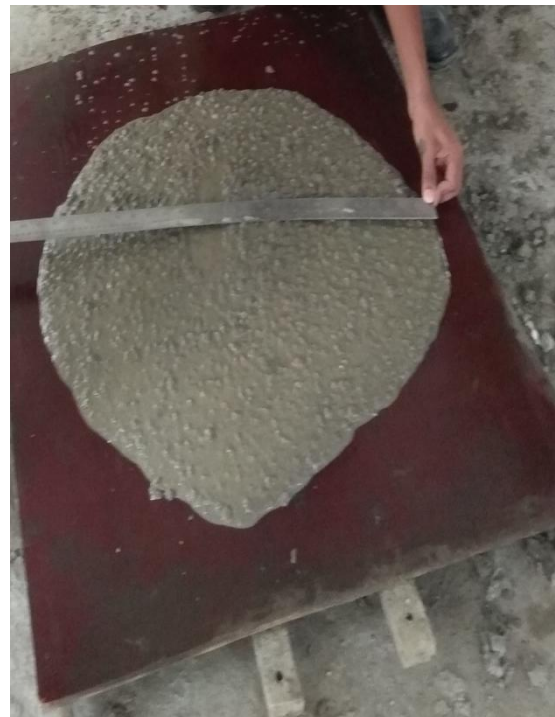
Figure 5. Slump Flow Spread
