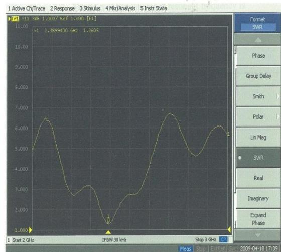
Figure 13 SWR pattern of the antenna designed – Network analyzer
