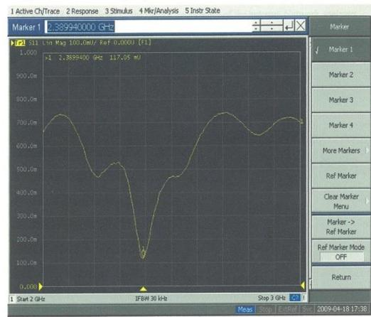
Figure 11 Resonant frequency of the antenna on Network analyzer
