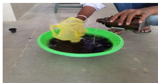
Fig.4: Cleaning of hair with acetone
