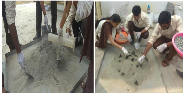
Fig.5: Preparation of concrete mix with addition of Hair fibre
