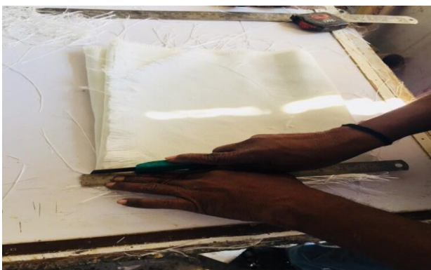
Fig:2 Cutting of Glass Fiber
