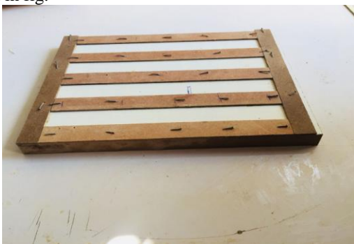
Fig:1.Wooden Mould to arrange composite material
