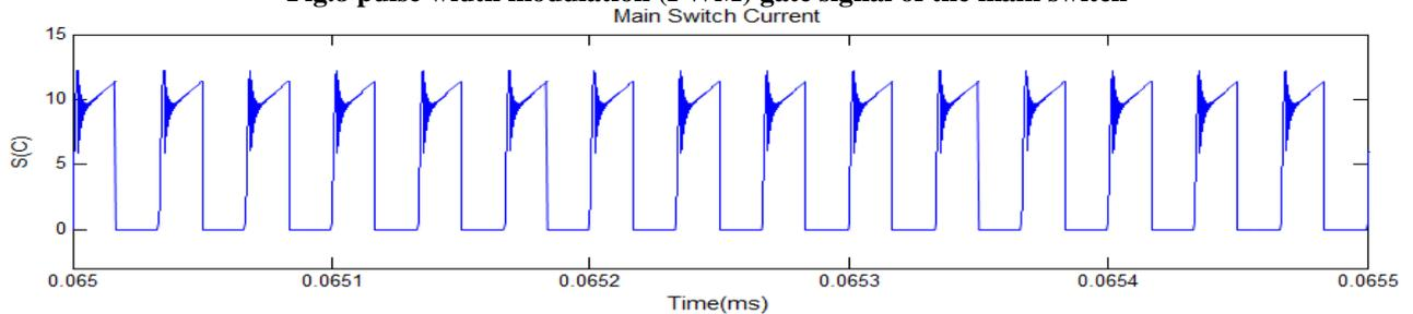
Fig.9 Current of the main switch
