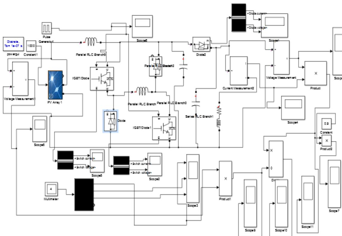
Fig.6 Soft switching boost converter using R-load.
