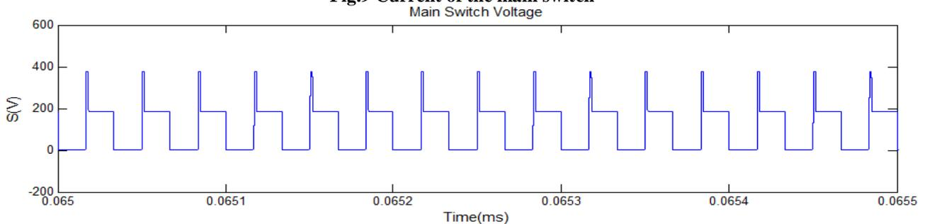
Fig.10 Voltage of the main switch
