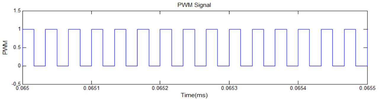
Fig.8 pulse width modulation (PWM) gate signal of the main switch
