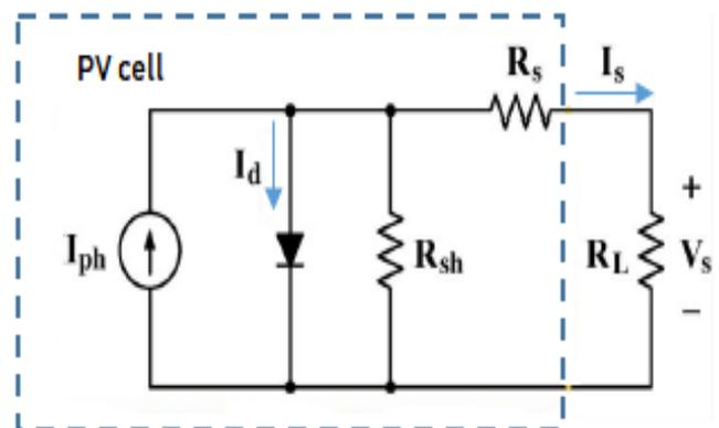
Fig.1 Equivalent circuit of a PV cell.
