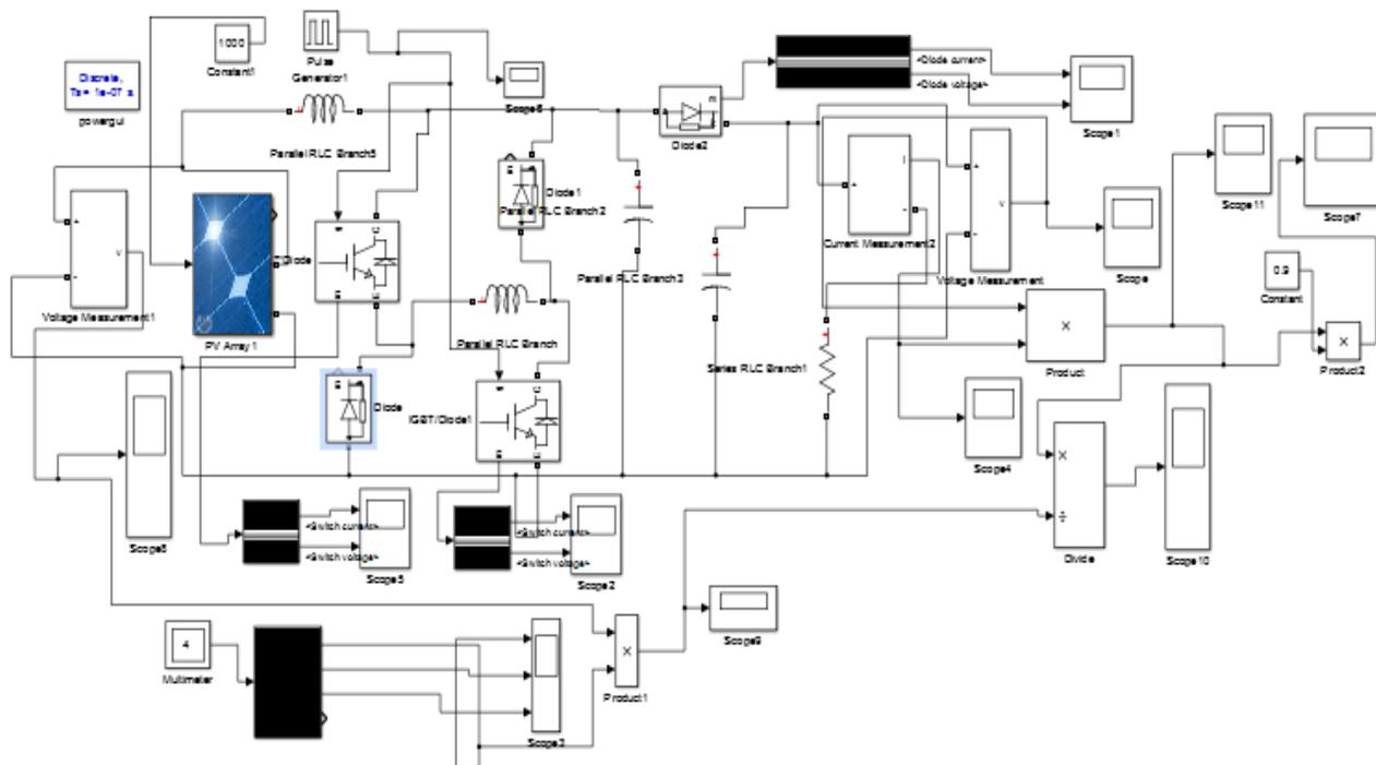
Fig.5 Soft switching boost converter using R-load
