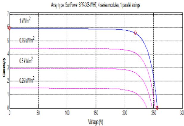
**Fig.2 V-I characteristics curves at different irradiance and 25oC**
