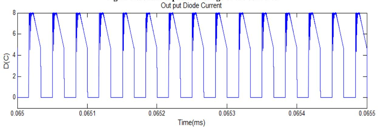
**Fig.13 Output diode current of the soft switching boost converter**
