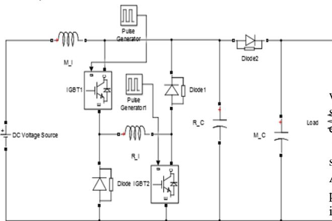
**Fig. 3. Circuit diagram of soft-switching boost converter.**
