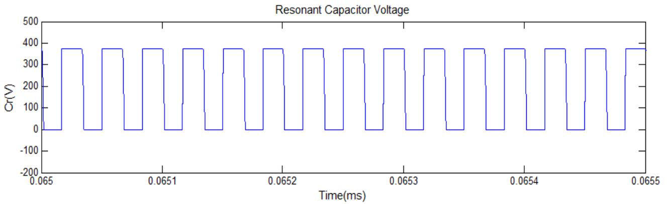
**Fig.12 Resonant capacitor voltage of the converter**
