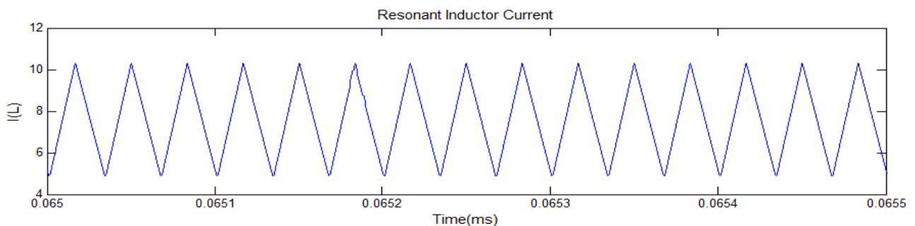
Fig.11 Resonant inductor current of the converter
