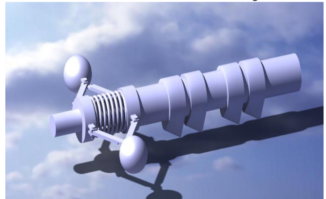
Fig 1: Inlet Camshaft Full Link Model
