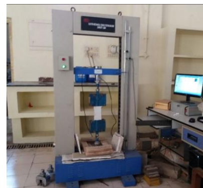
Fig 3: Testing of dog-bone shaped specimen under uni-axial tension
