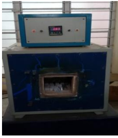
Fig 3 (C) Electric Furnace with inert gas set up
