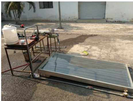
Figure 2 Experimental setup of solar collector
