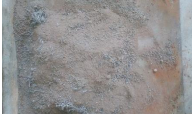
Figure 2: Dry mix of soil, cement and steel scrap
