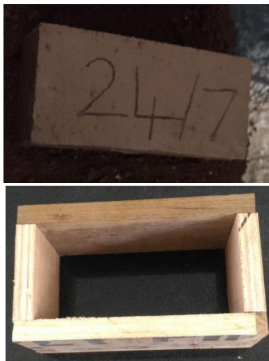
Figure 3: Production of bricks using wooden mould
