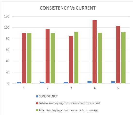
Fig. 4.4 Consistency Vs Current for before and after employing consistency control in ODL stage
