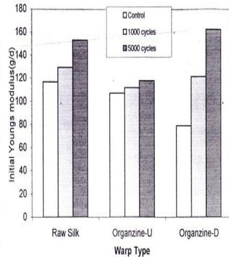
**Fig 3 Comparison Of Initial Young's Modulus For The Three Warp Types**
