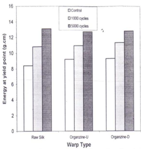
**Fig 2 Comparison Of Energy At Yield Point For The ThreeWarp Types**
