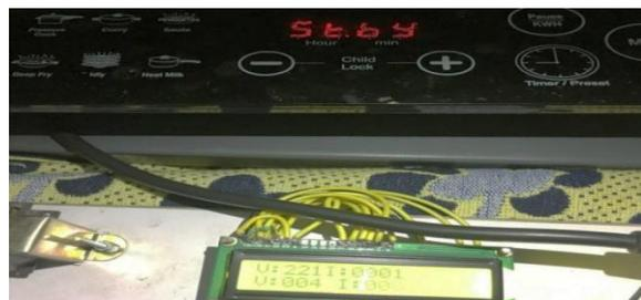
Fig.10. Current reached zero during standby load
