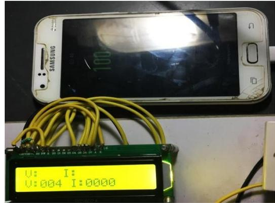
Fig.8. Mobile goes to cut off stage @ 100% SoC
