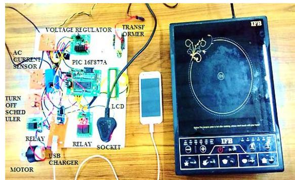
Fig.9.Implementation of Smart Socket
