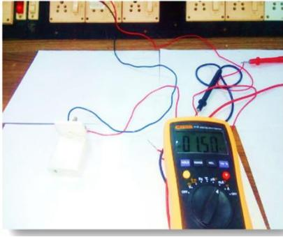
Fig.2. Consumption of current by mobile phone from mains
